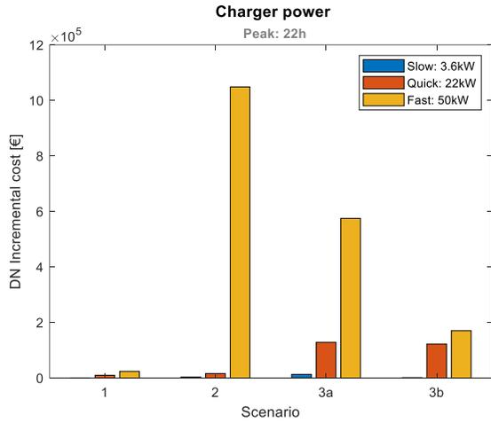
Fig. 12. Dependence of distribution network incremental costs with charging power level for each scenario.
