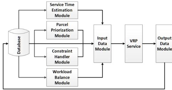
Fig. 3. Functional scheme of the route optimization model.
