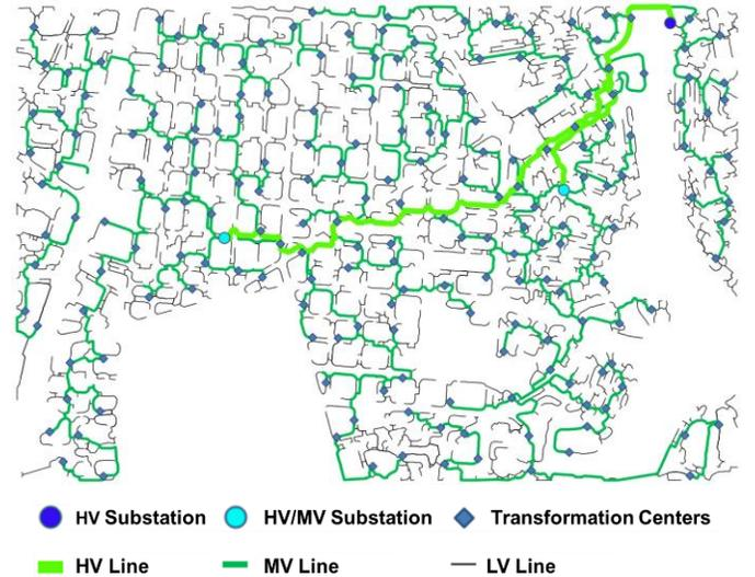
Fig. 9. Base case distribution network for the area of PSH 1.
