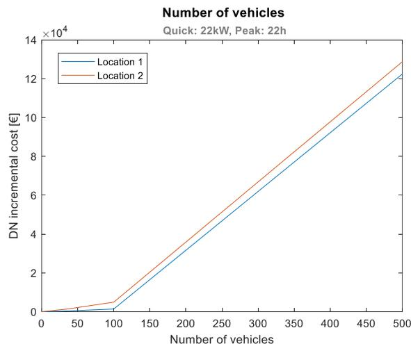
Fig. 11. Dependence of distribution network incremental costs with the number of electric vehicles at locations 1 and 2.
